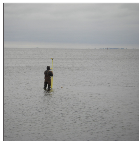
Collecting elevation data in North Carolina tidal flats using survey grade Real-Time Kinematic GPS instruments.
