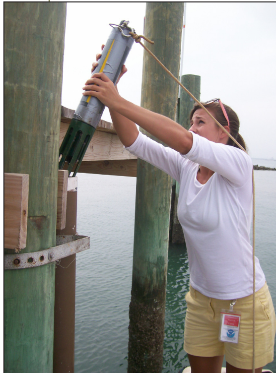
Placing a water quality and depth data sonde for the NERRS System-Wide Monitoring Program (SWMP) in North Carolina. SWMP data can be used to augment tidal wetland reference site data at NERR sites.
